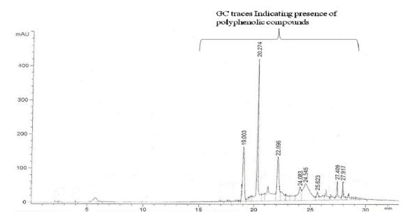
Figure 8. HPLC traces acquired with a reversed-phase gramin C-18 column 150 x 4.60 mm; particle size, 5 μm; temperature, 40 °C; injection volume, 10 μL, DAD λ, 254 nm and gradient system; specifically set for detection of polyphenolic content in the ethanol extract of the root bark of *Synadenium glaucescens*
