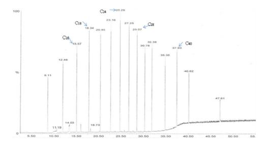
Figure 1. GC traces for a C12-C60 Standard
